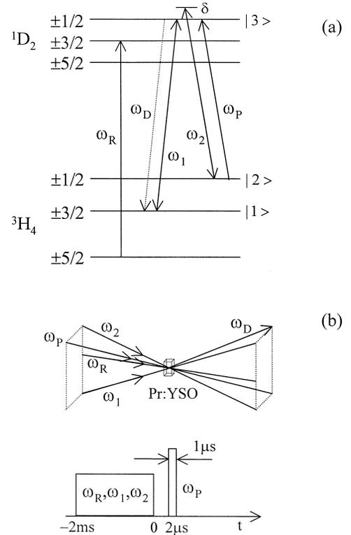
Fig. 1. (a) Energy level diagram of Pr:YSO and (b) laser beam propagation scheme and pulse sequence for phase-correlated four-wave mixing spectroscopy.
