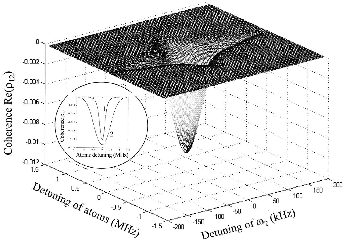
Fig. 4. Numerical simulation for the Raman excited spin coherence  $\text{Re}(\rho_{12})$  vs. atoms detuning and two-photon detuning  $\delta$  for solid curve in Fig. 3. Inset:  $\text{Re}(\rho_{12})$  vs. atoms detuning for zero detuning of  $\omega_2$ , and  $\Omega_2 = 5\Omega_1$ , where  $\Omega_i$  is Rabi frequency of curve  $i$ .
