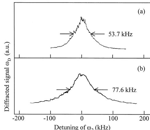
Fig. 2. Four-wave mixing signal  $\omega_D$  vs. two-photon detuning  $\delta$  with (a) unstabilized and (b) stabilized lasers.
