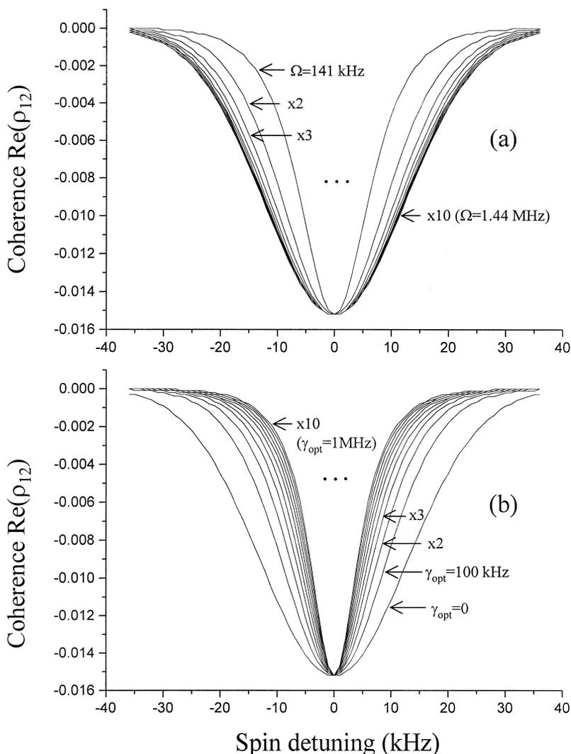
Fig. 6. Numerical simulation for the Raman excited spin coherence  $\text{Re}(\rho_{12})$  vs. spin distribution. Optical transition is assumed to be homogeneously broadened. (a) Optical homogeneous decay rate  $\gamma_{\text{opt}} = 100$  kHz and (b)  $\Omega_1 = \Omega_2 = 200$  kHz.
