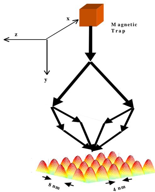
Figure 4. Basic illustration of the steps involved in producing two dimensional beam-splitting and recombining. For simplicity, the laser beams are not shown in the diagram. The two dimensional pattern at the bottom is produced via numerical simulation of the process described in the body of the text.
