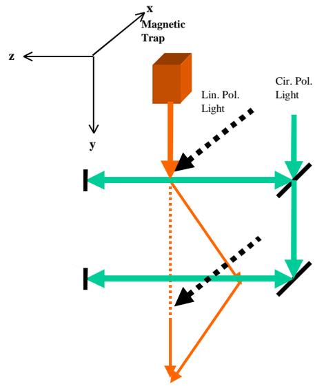
Figure 3. Schematic illustration of the three dimensional geometry employed in producing a beam splitter and recombiner via adiabatic following in the Raman dark state.
