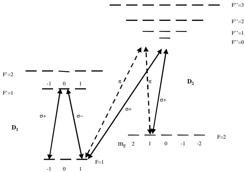
Figure 1. Schematic illustration of the relevant energy levels of  $^{87}\text{Rb}$  atoms, considered in this article as an example. Transitions from both the  $D_1$  and the  $D_2$  manifolds are used. The presence of two different types of Raman transitions in the  $D_2$  manifold, excitable by optical beams propagating in orthogonal direction, is a key element of this design.
