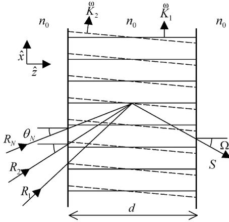
Fig. 2. Schematic illustration of the combination of  $N$  mutually incoherent input beams into a single output beam.
