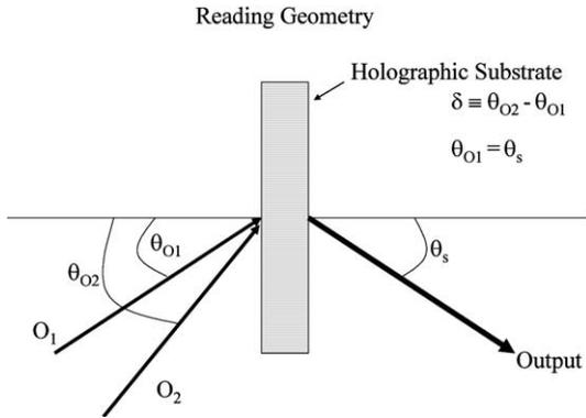
Fig. 4. Illustration of the geometry for reading the two holograms, the first one ( $O_1$ ) at 980 nm and the second ( $O_2$ ) at 980 nm +  $\Delta\lambda$ . Both beams will be diffracted at the same exit angle,  $\theta_s$ .
