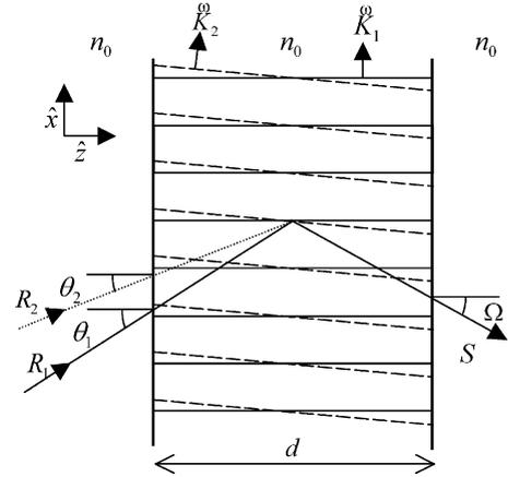
Fig. 1. Schematic illustration of the combination of two mutually coherent input beams into a single output beam.
