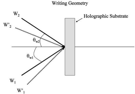
Fig. 3. Schematic illustration of the geometry for writing two holograms at 514.5 nm. The angles of the writing beams are chosen to ensure that when the holograms are read by lasers at 980 nm, the output beams overlap.
