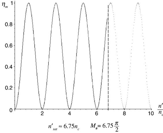
Fig. 5. Schematic illustration of the functional dependence of the optimal (i.e., Bragg-matched diffraction efficiency) as a function of the index modulation amplitude and  $M_{\#}$ . See text for details.
