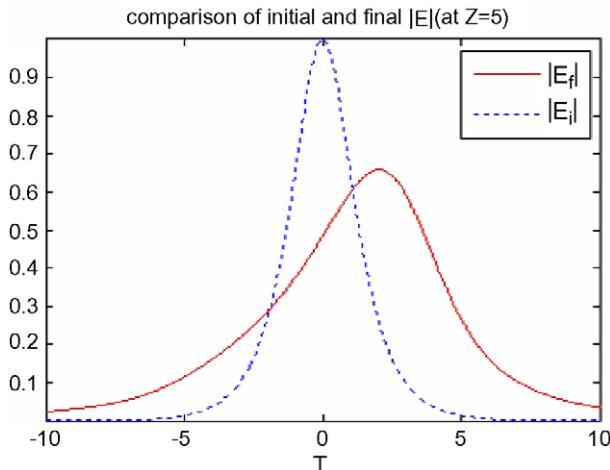
Fig. 9. Pulse spreading in non-instantaneous Kerr medium ( $\tau = 1$ ) with the initial field  $|E_i|$  and the final field,  $|E_f|$ .
