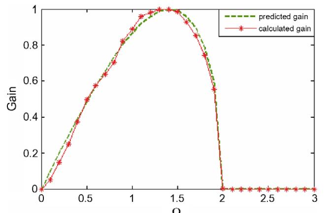
Fig. 1. Gain spectrum for the instantaneous nonlinear Kerr medium.
