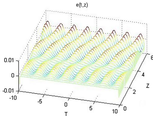
Fig. 2. Gain of the periodic temporal perturbation versus propagation distance. Perturbation parameters:  $\varepsilon = 0.001$  and  $\Omega = 2.5$ .
