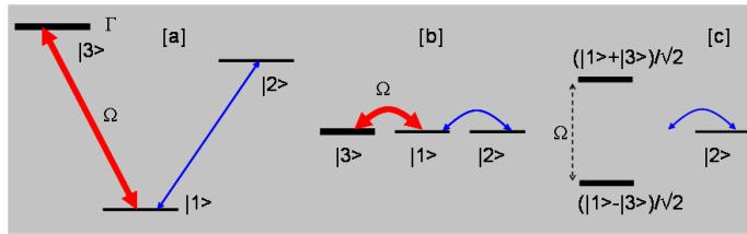
Fig. 1. The quantum Zeno effect for atomic transitions. The state  $|1\rangle$  is weakly coupled to  $|2\rangle$ , but this evolution is continuously suppressed by the presence of a pump laser coupling  $|1\rangle$  to  $|3\rangle$ .
