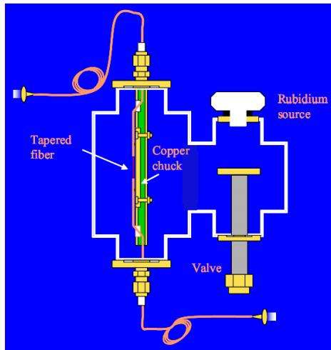
Fig. 2. Schematic of the tapered Nano fiber set-up
