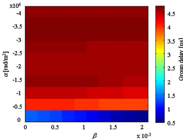
Fig. 5. Minimal group delay in the LCBG reflection band. The grating length is 2 mm and the center wavelength is 1.52  $\mu\text{m}$ .
