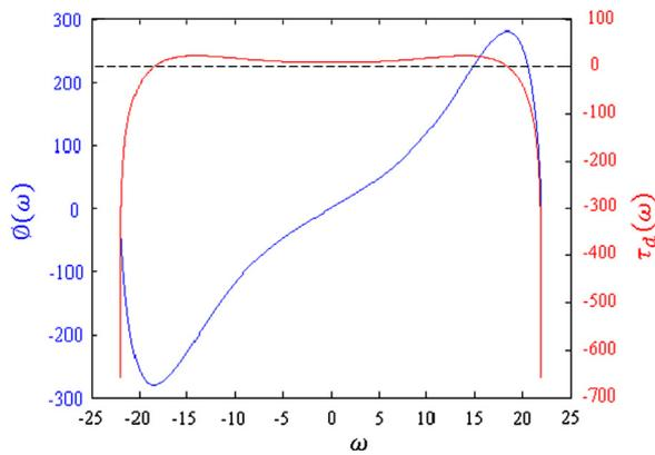
**Fig. 10.** Phase response (blue) and the corresponding group delay (red) of a generic minimal phase bandpass filter centered at  $\omega=0$ . (For interpretation of the references to color in this figure legend, the reader is referred to the web version of this article.)
