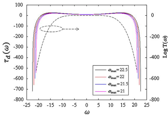
**Fig. A1.** Dependence of the group delay calculated by the Hilbert transform of the frequency calculation window. Dashed black—log plot of the amplitude transfer function of the filter.
