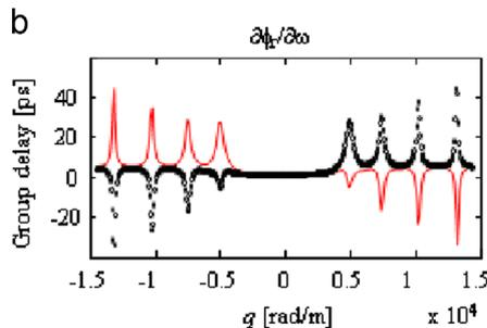
Fig. 6. Reflection (a) and group delay of LCBG calculated by TMM. Red solid line:  $\alpha < 0$ , dashed line:  $\alpha > 0$ . The parameters are identical to those used for Fig. 4. (For interpretation of the references to color in this figure legend, the reader is referred to the web version of this article.)
