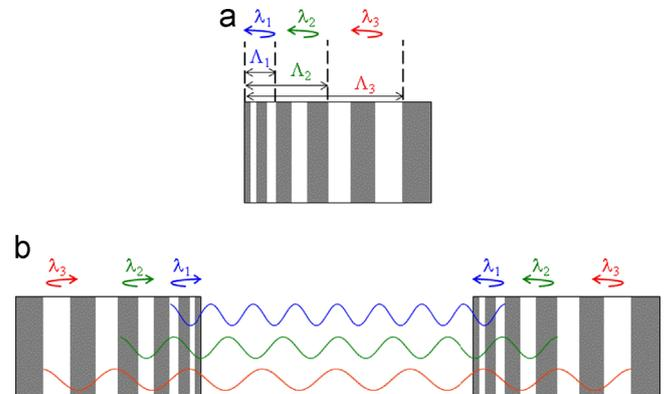
Fig. 2. LCBG based WLC realization: (a) three different wavelengths ( $\lambda_1 < \lambda_2 < \lambda_3$ ) are reflected at different locations inside the grating region, (b) schematic illustration of a Fabry–Perot (FP) cavity of length  $L$  formed by a pair of LCBGs.
