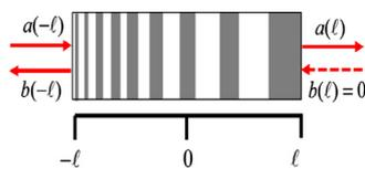
Fig. 3. Field propagates along  $z = -l \sim l$ .  $a(-l)$  and  $a(l)$  are the input and the transmitted field, respectively.  $b(-l)$  is the reflected field.
