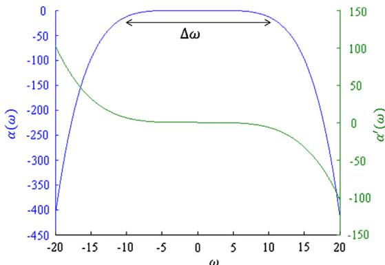
Fig. 8.  $\alpha$  (blue) and the corresponding  $\alpha'$  (green) of a generic minimal phase bandpass filter centered at  $\omega=0$ . (For interpretation of the references to color in this figure legend, the reader is referred to the web version of this article.)
