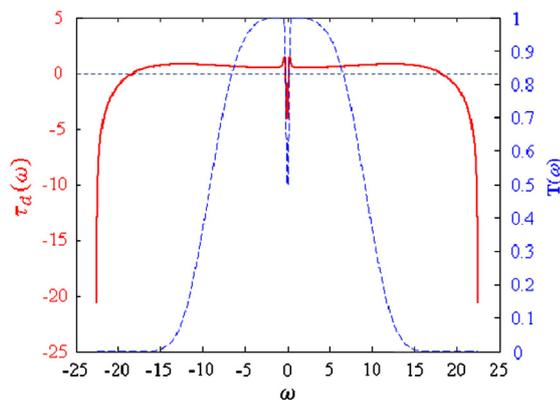
**Fig. 11.** Group delay (red) and amplitude transfer function (blue) of a flat-top filter incorporating a notch at the center of its pass-band. (For interpretation of the references to color in this figure legend, the reader is referred to the web version of this article.)
