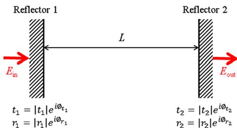
Fig. 1. Schematic illustration of FP cavity based WLC.
