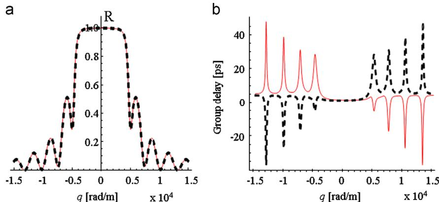
Fig. 4. Reflection (a) and group delay (b) of LCBG calculated according to Eq. (4a). Red solid line:  $\alpha < 0$ , dashed line:  $\alpha > 0$ . The parameters are defined in the text. (For interpretation of the references to color in this figure legend, the reader is referred to the web version of this article.)
