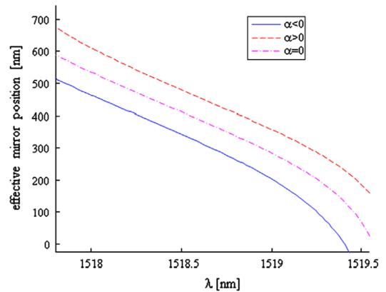
Fig. 7. Effective mirror position with respect to the grating edge within the reflection bandwidth of the LCBGs. Dash-dot magenta—no chirp, dashed red—positive chirp, solid blue—negative chirp. The gratings parameters are as in Figs. 4 and 6. (For interpretation of the references to color in this figure legend, the reader is referred to the web version of this article.)
