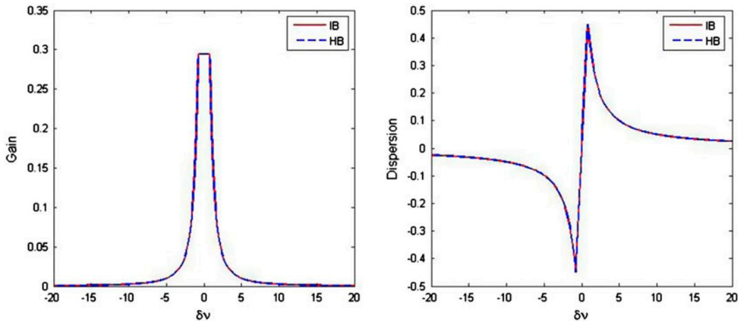
Figure 6. Effective gain and dispersion in the homogeneous (dashed lines) and inhomogeneous (solid lines) broadening cases, in a single mode laser cavity.  $\sigma = 0.1$  MHz,  $\Gamma = 1$  MHz,  $G = 1$ ,  $Q = 0.0252$ . (The color version of this figure is included in the online version of the journal.)
