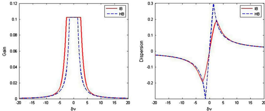
Figure 7. Effective gain and dispersion in the homogeneous (dashed lines) and inhomogeneous (solid lines) broadening cases, in a single mode laser cavity.  $\sigma = 2$  MHz,  $\Gamma = 1$  MHz,  $G = 1$ ,  $Q = 0.0252$ . (The color version of this figure is included in the online version of the journal.)
