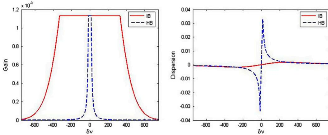
Figure 5. Effective gain and dispersion in the homogeneous (dashed lines) and inhomogeneous (solid lines) broadening cases, in a single mode laser cavity.  $\sigma = 300$  MHz,  $\Gamma = 1$  MHz,  $G = 1$ ,  $Q = 0.0252$ . (The color version of this figure is included in the online version of the journal.)
