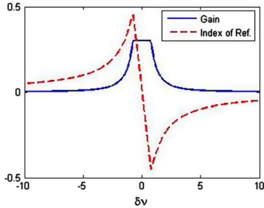
Figure 1. Homogeneous gain (solid line) and dispersion (dashed line) in a laser under steady state operation. (The color version of this figure is included in the online version of the journal.)
