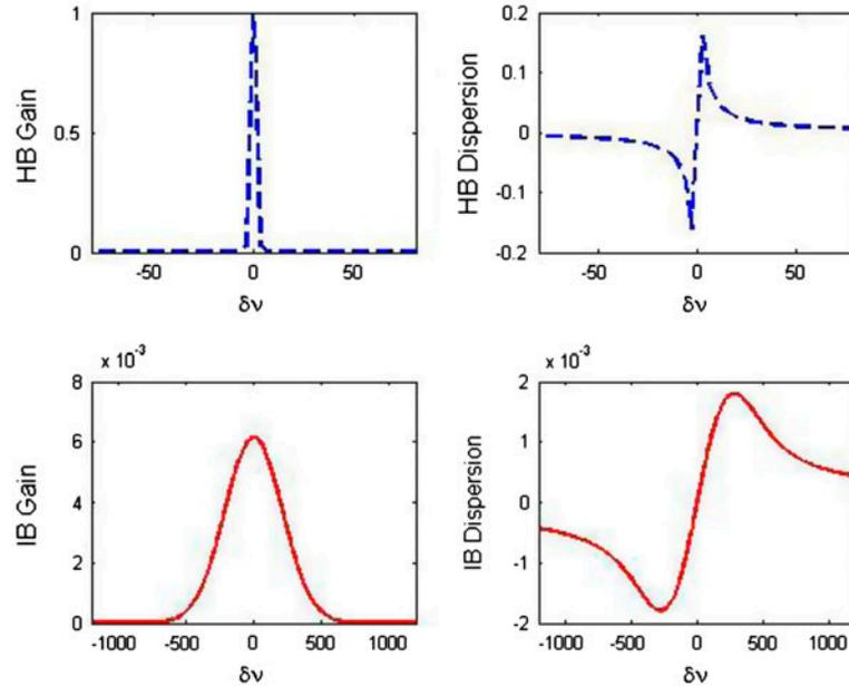
Figure 3. Effective gain and dispersion in the homogeneous (dashed lines) and inhomogeneous (solid lines) regimes, in free space.  $\sigma = 300$  MHz,  $\Gamma = 1$  MHz,  $G = 1$ ,  $Q = 0.0252$ . (The color version of this figure is included in the online version of the journal.)
