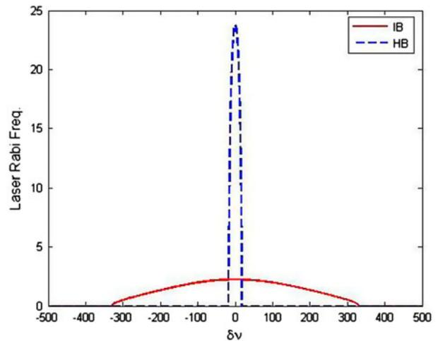
Figure 4. Homogeneously (dashed line) and inhomogeneously (solid line) broadened laser Rabi frequencies,  $\Omega$ .  $\sigma = 300$  MHz,  $\Gamma = 1$  MHz,  $G = 1$ ,  $Q = 0.0252$ . (The color version of this figure is included in the online version of the journal.)
