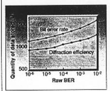
New holographic recording schedule developed at IBM involves maintaining the bit error rate (BER; top curve) rather than the diffraction efficiency (bottom curve). This allows considerably more holograms to be recorded (M) in the same volume.
