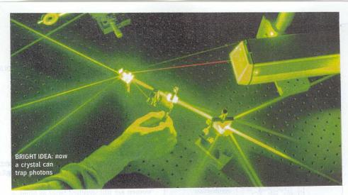
lattice of yttrium silicate doped with ions of the metal praseodymium. Using a laser beam—called the coupling beam—they tuned the praseodymium ions to put their electrons into a "dark" state. In this state they were unable to jump to higher energy levels and so could not absorb light of a particular wavelength. They then sent a second beam of that wavelength into the solid.
